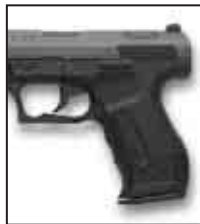
TRIGGER IN FORWARD POSITION FOR SINGLE AND DOUBLE ACTION FIRING
